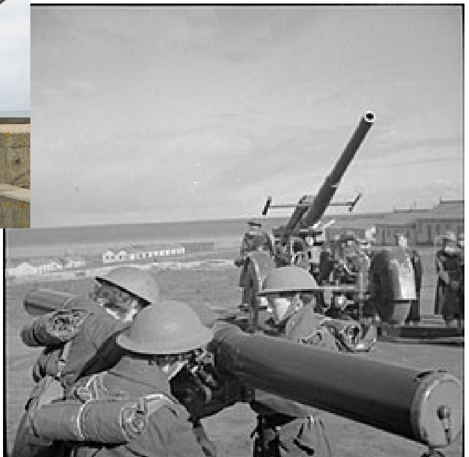
ATS women operate a rangefinder at Weybourne Camp on 23 rd October 1941 in front of mobile 3.7 inch AA gun
